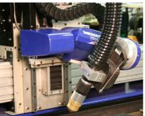
**BEVEL-R® 5-AXIS, COMPACT** PLASMA BEVEL UNIT WITH SURESTOP COLLISION SENSOR Low profile plasma bevel head with 360° programmable rotation with no cable or torch lead wind up rapidly processes your weld prep parts. SureStop Collision Sensor for guick, simple torch realignment. (Optional)
