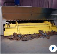
**THE SLAGGER® TABLE** The standard Slagger<sup>®</sup> unitized construction cutting table is a selfcleaning, side-draft zoned and ducted table with easy cleaning and small parts retrieval. With optional downdraft table
