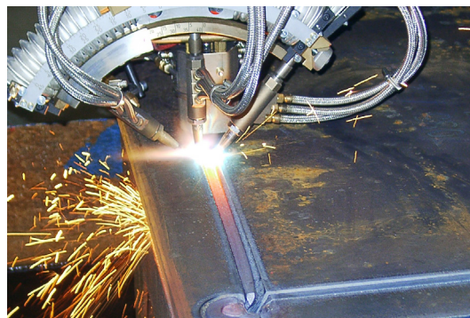
DAF/L Cutting a K Bevel
