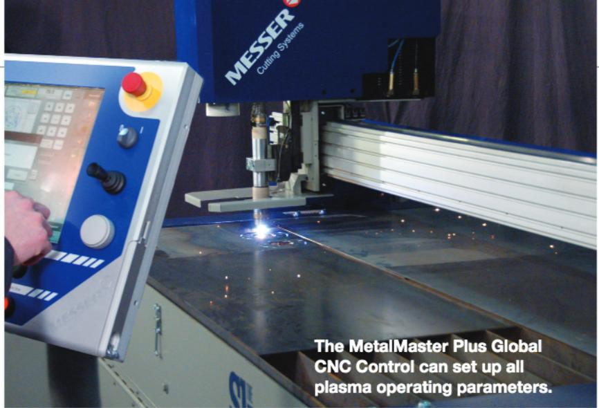
**The MetalMaster Plus Global CNC Control can set up all plasma operating parameters.**
