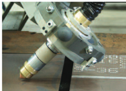
The bevel angle is set automatically using a combination of A-axis and C-axis interpolation by the CNC.
