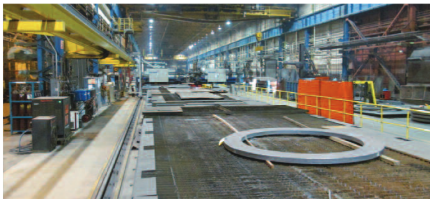
Most of the steel Holtec Manufacturing uses is initially cut on one of two 100-foot-long Messer Cutting Systems cutting tables.
