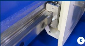
**LINEAR WAYS** Precision linear ways with ball runner blocks in the Y-Axis.
