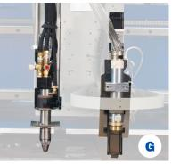
PLASMA AND OXYFUEL TORCHES SL-200, SL-300 AND PL-1 LIFTERS Plasma and oxyfuel torches for precision cutting. Supported by the SL Series Oxyfuel Lifters and PL-1 Plasma Lifters provide a smooth and rigid platform for vertical cutting to minimize non-productive time. (Optional)
