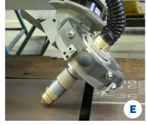
**GLOBAL INFINITY ROTATOR** Unique compound skew control of A & C-Axis is automatically positions the torch. Cut edges of +45° through -45° with automatic torch height control via arc voltage. Square corners are achieved utilizing custom looping routines. Bevel angle change-on-the-fly (BACF) is available to generate transition angular edges. (Optional)
