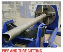
Plasma bevel and vertical cutting of pipe and tube from 2 to 24" diameter. Length up to 40' maximum. Cut up to ¼"-1¼" wall thickness. Offline software provided by specialists in 3D pipe and tube profiling. (Optional)
