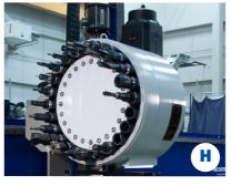
4"DRILL AND 24 POSITION ROTARY TOOL CHANGER
