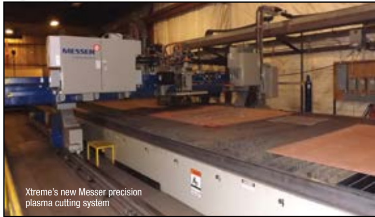
Made in-house, these racks are drop in replacements. Combined with the Messer’s built in slag removal system, downtime is minimized
