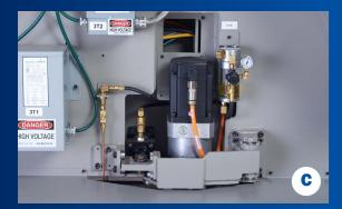
Powerful, precise, 21 HP drives for the X and Y-Axis, provide smooth accurate motion for excellent cut quality,
