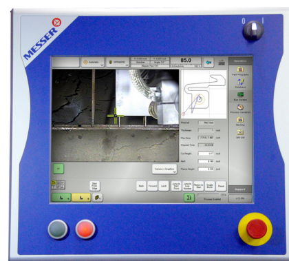
Video camera featured (right) allows for fast, accurate plate alignment.
