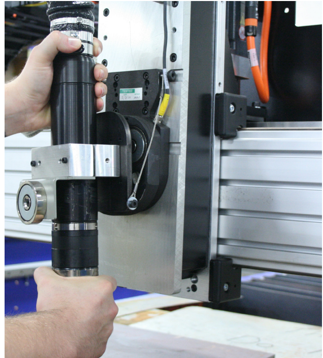
Surestop Collision Sensor with quick and accurate reset.
