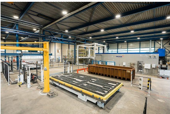
Caption: "Solutions Beyond Machines" at Joop van Zanten (Netherlands) with Messer Cutting Systems PowerBlade with fiber laser technology and OmniMat with plasma bevel cutting, OmniFab digitalization solution, OmniWin CAD/CAM software, and material handling system. © Messer Cutting Systems
