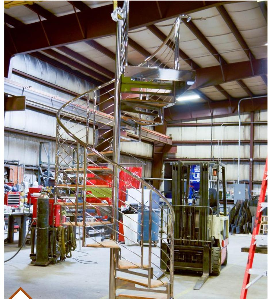
*The need to process large volumes of stainless steel and aluminum, such as the stainless steel staircase shown here, was in part why Lyman-Morse ultimately chose the XPR300 with X-Definition Plasma.*
