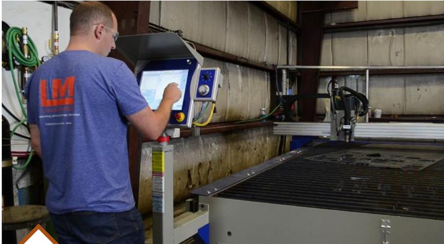
*Lyman-Morse's XPR300 was integrated into a system designed and built by Messer Cutting Systems. The system features a Messer MetalMaster Evolution gantry that is attached to Messer's Slagger cutting table.*
