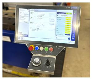
The **Global Connect L** (Lite) featured on the MetalMaster 3.0 with the optional 8-position joystick and handwheel/feedrate.
