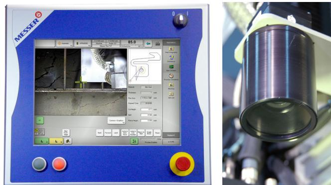
Video camera featured (right) allows for fast, accurate plate alignment.
