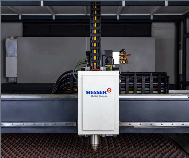
Protected cutting head and guide-ways.
